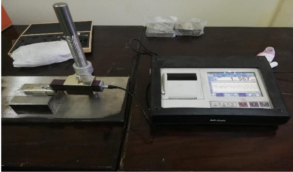
Fig. 2. Surf test Mitutoyo Sj-310 Device While Measure Surface Roughness.
