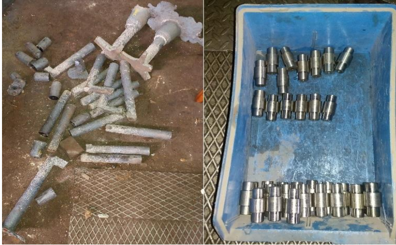
Fig. 1. Casting and Machining Samples for Manganese Steel
