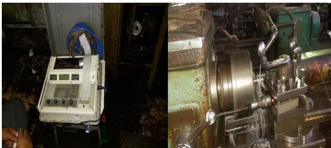
Mechanalysis Model 880 Device While measuring Vibration
